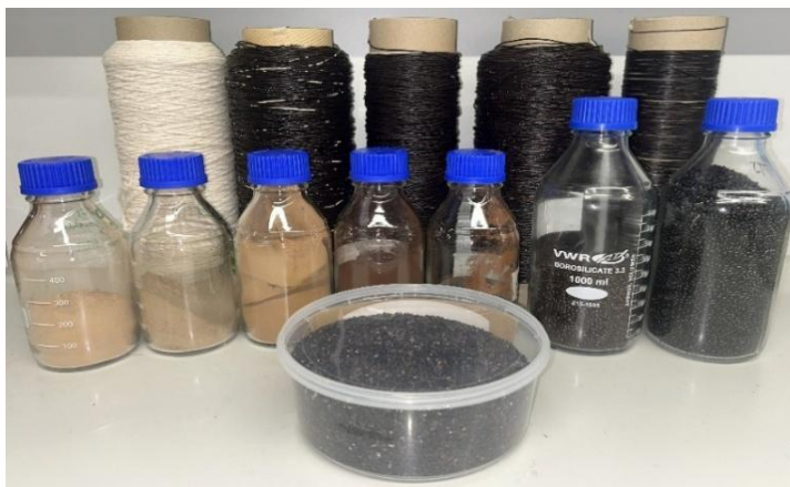
Lignins are available in various qualities. Only a few are suitable for spinning fibers or for coating yarns and textiles. ©DITF
